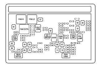
The underhood fuse block is located in the engine compartment, on the driver side of the vehicle. Lift the cover for access to the fuse/relay block.
